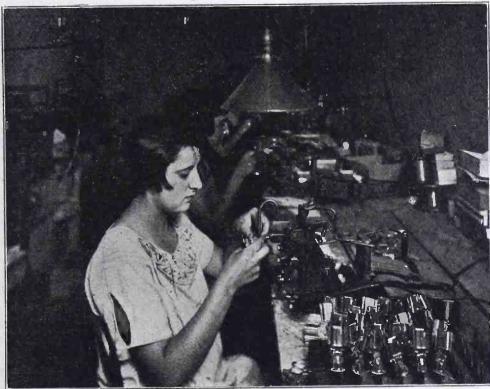
Electric spot-welding plates and grids onto their supporting wires. The weld is made by a low-voltage, high-amperage arc. Note the rack full of completed stems in the foreground. These are ready for sealing into bulbs.
